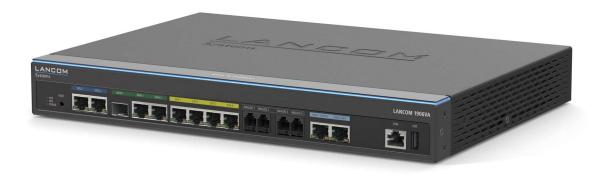
Dual-VDSL VPN router with two integrated VDSL modems for up to 200 Mbps – ideal for load balancing and professional telephony
